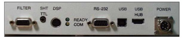
Figure 10. Cable Connections (Back Panel)
